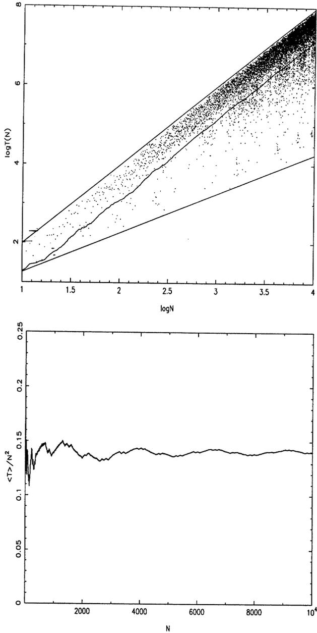
Fig. 6. – Maximal period of the orbits, on a lattice of size  $N$ , for the golden mean rotation number. *Top*: the period function  $T(N)$ , with upper and lower envelopes, and its average order  $\langle T \rangle$ . *Bottom*: normalized average order  $\langle T(N) \rangle / N^2$ .
