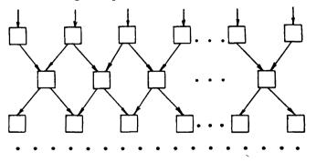
The processors are indicated by squares and the flow of information by arrows. The input word is fed, letter by letter, to the processors in the top row. The output of each processor depends only on its current inputs. The final
